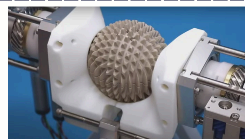
Figure 1 ABENICS: Active ball joints (4)
